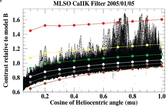
$$\bar{I}_{m,\mu}(\lambda_0) = \int I_{m,\mu}(\lambda_0) \Phi(\lambda - \lambda_0) d\lambda \begin{cases} I_{m,\mu} = \text{ The m}^{\text{th model intensity.}} \\ \Phi(\lambda) = \text{ Instrument bandpass profile.} \\ \mu = \cos(\theta), \theta = \text{heliocentric angle.} \end{cases}$$
