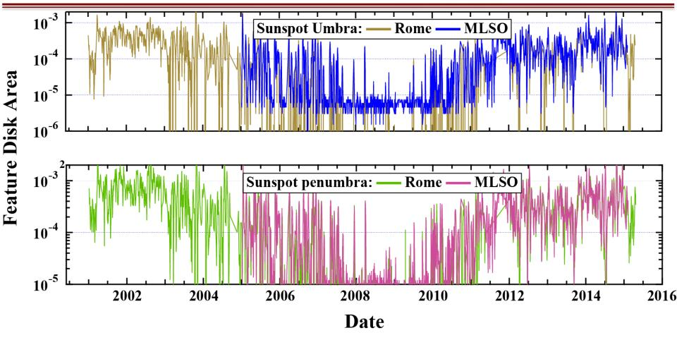
• Dead pixels in MLSO leave a persistent sunspot area of ~8x10<sup>-6</sup> making an irradiance offset of <0.0008 Wm<sup>-2</sup>nm<sup>-1</sup> in the MLSO data. Will correct MLSO irradiance to match Rome value in the combined data set.
