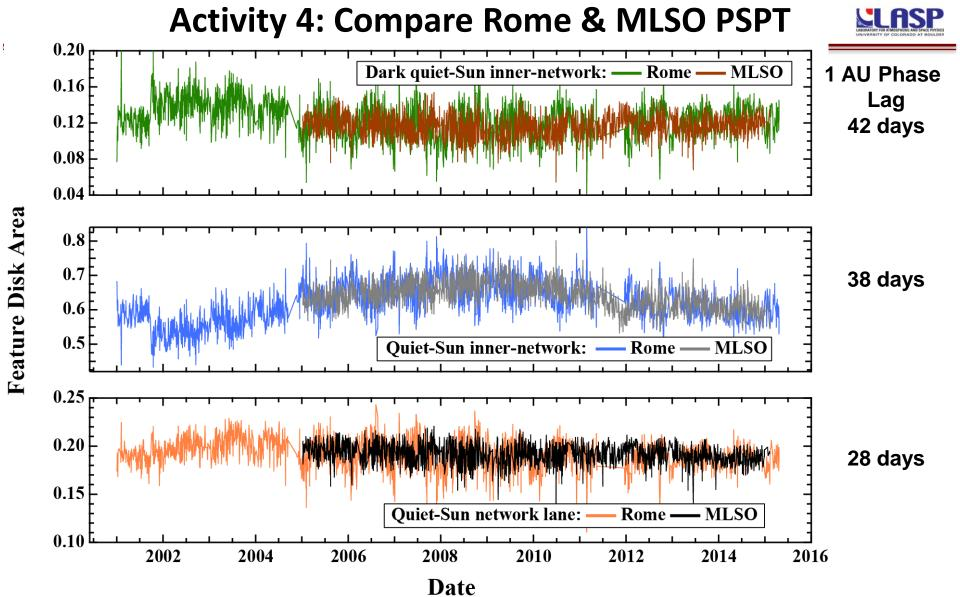
Small quasi-annual oscillation in quiet-Sun data – presumably due to slight defocus in telescope (?); problem less apparent in MLSO data; not coherent with 1 AU
